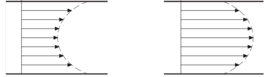
Figure 4. Steady, stable fluid flows in a channel [3].
