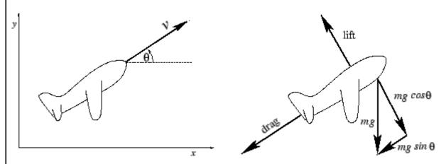
If we apply Newton's second law of motion (force =  $mass \times acceleration$ ) and examine the major forces acting on the plane, we see easily the force acting in the forward direction of the plane is
