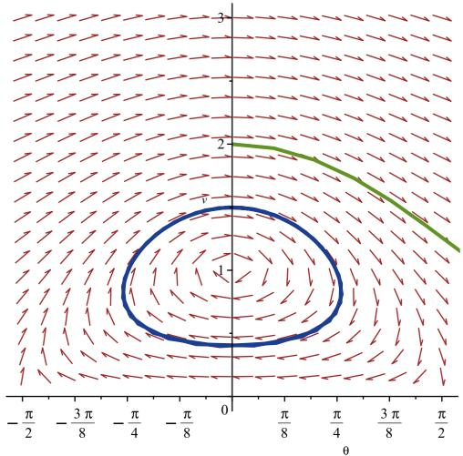
> DEplot(phug, [theta(t),v(t)], t=0..10, [[theta(0)=0, v(0)=1.5], [theta(0)=0, v(0)=2], [theta(0)=0, v(0)=1.05]], theta=-Pi/2..3\*Pi, v=0..3, tickmarks=[piticks,default])
