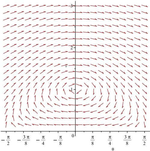
> DEplot(phug, [theta(t),v(t)], t=0..10, [[theta(0)=0, v(0)=1.5], [theta(0)=0, v(0)=2]], theta=-Pi/2..Pi/2, v=0..3, tickmarks=[piticks,default])
