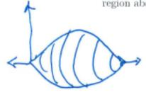
AT A TYPICAL X VALUE, A CROSS SECTION IS A DISK
