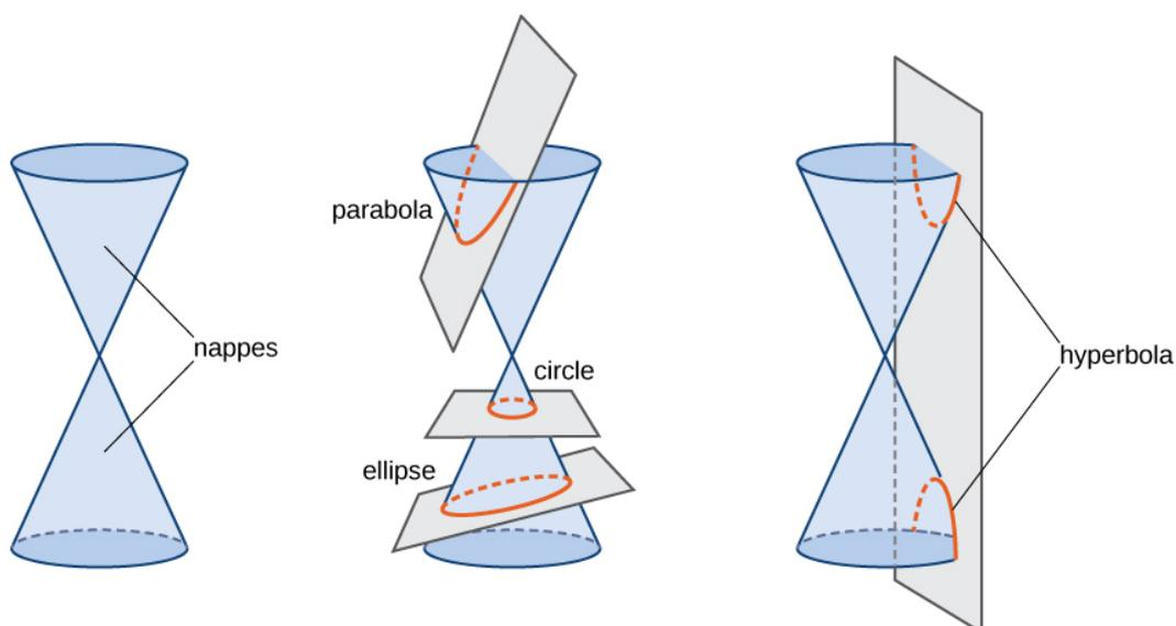
**Figure 7.44** The four conic sections. Each conic is determined by the angle the plane makes with the axis of the cone.
