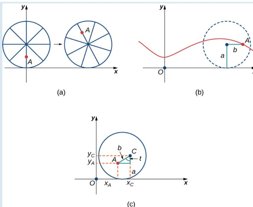
**Figure 7.14** (a) The ant climbs up one of the spokes toward the center of the wheel. (b) The ant's path of motion after he climbs closer to the center of the wheel. This is called a curtate cycloid. (c) The new setup, now that the ant has moved closer to the center of the wheel.
