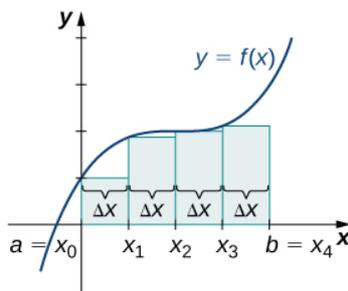
**Figure 1.8** With a left-endpoint approximation and dividing the region from  $a$  to  $b$  into four equal intervals, the area under the curve is approximately equal to the sum of the areas of the rectangles.
