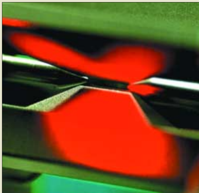
Ions can be entangled using a linear chain of them that have been trapped in the electric field between a pair of elongated electrodes. This photo shows the experimental set-up used to trap calcium ions at the University of Innsbruck.
