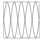
These vibrations make tones which are multiples of the fundamental tone. They sound higher than the fundamental tone; they are called "overtones" of the fundamental.
