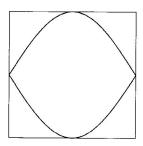
This makes a sound which we call the "fundamental tone"; it is the lowest note this length of string can produce. However, it can also vibrate with 3 or with 5 humps:
