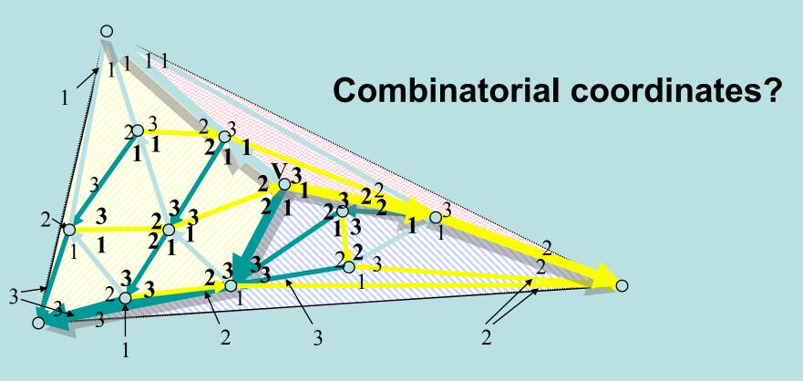
Count triangles in each partition of the 3-partition of the triangulation, then divide the count by the total number of internal triangles, and interpret the value as barycentric coordinates on three affinely independent points.
