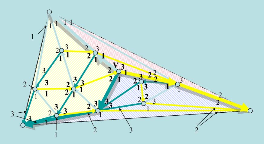
The three different colored paths from V to the three extreme triangle vertices partition the triangle set into three disjoint subsets of the [2n–5] interior triangles
