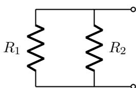
Given:  $R_{\text{total}} = 2$ ,  $R_2 = R_1 + 3$ .
