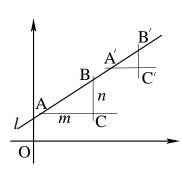
Let m be the line through A parallel to x-axis (exists and is unique by Parallel lines axiom), and n the line through B parallel to y-axis. By Exercise 9.1,  $m \perp n$ . Let C be the intersection point of m, n. Then  $\triangle ABC$  is the right triangle:  $m \angle C = \pi/2$ , and  $|AC| = x_2 - x_1$ ,  $|BC| = y_2 - y_1$  where  $A = (x_1, y_1), B = (x_2, y_2)$ .
