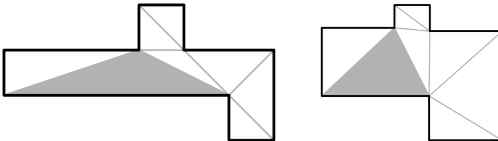
FIGURE 2. Two compatible triangulations of different polygons. The most distorted triangle is shaded; this determines an upper bound for the piecewise linear map between the polygons.
