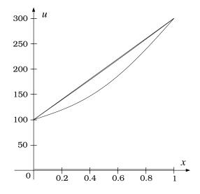
Notice that there is very little distinction between the graphs of u(x, 0.5) and  $u(x, \infty)$ . So in just 0.5 sec, the distribution of temperature in the rod is almost equal to the steady-state temperature.
